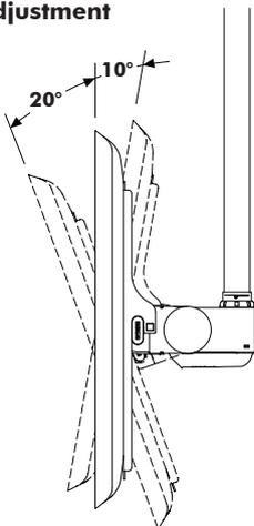
**NOTE:** To achieve the maximum 20° downward tilt, THE MAXIMUM HEIGHT OF A DISPLAY IS 1143mm (45").
